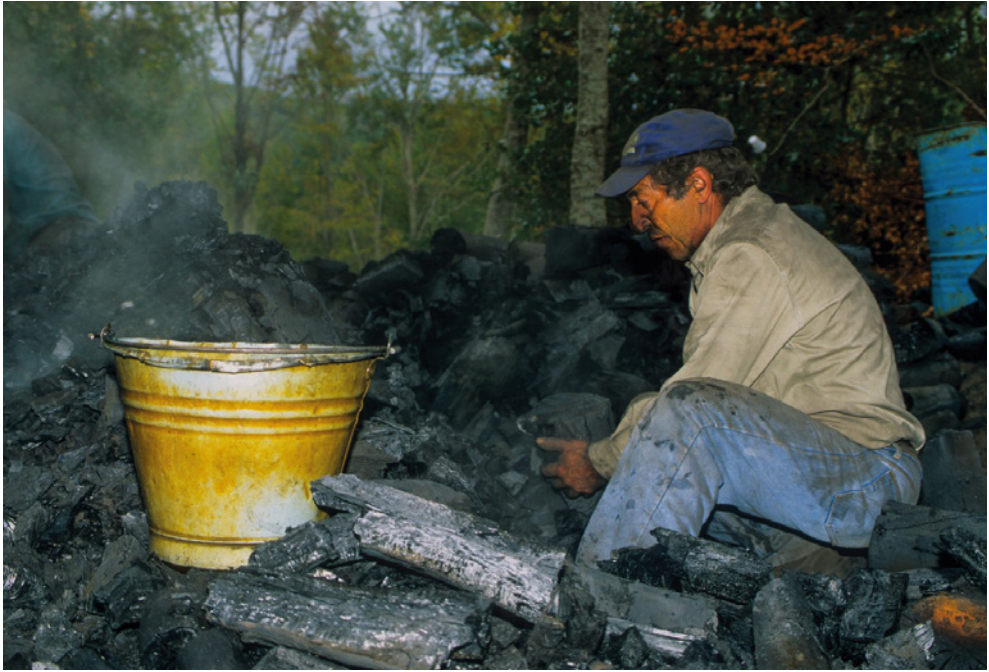
Fig. 5. Separation of finished product from insulating soil (credits: ©Gino Fabio, 2001)
